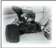
Snow Blower - 35" Wide - 2 Stage - Hydraulic Drive - Adjustable Spout
