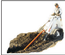
Trencher - 24" Cutting Depth 4" to 6" Chain Widths
