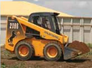
**ENHANCED STABILITY** ▲ with a wider tread width, low center of gravity, and increased machine width.
